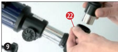
Be sure that the entrance of the eyepiece (the end you look into) is facing straight upwards. This will make observation easier. Alternatively, loosen the clamp screws (21) on the eyepiece holder and turn the zenith mirror into this position.
