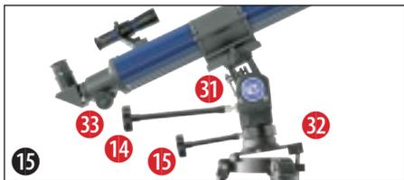
By turning both flexible shafts (14, 15) (Figure 1), the telescope can be moved horizontally and vertically.
