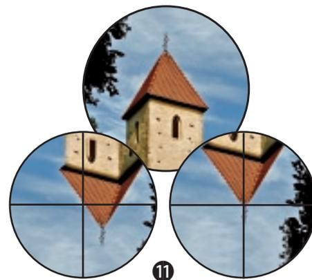
The image reproduced will be upright, but rotated around its vertical axis (you will see a mirror-image). In the finder, however, the reproduced image will be upright and its sides will not be reversed, as above. Now turn one of the two clamp screws (right/left) of the finderscope while looking continuously through the finder. Continue to turn until the finder's crosshairs are exactly over the position that corresponds to what you see when you look through the eyepiece of the main telescope.
