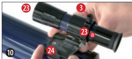
On the finder holder, there are adjusting screws for the finder (3) (Figure 1): two clamp screws (black) and one spring-loaded counter screw (silver). The clamp screws (black) are to be screwed (equally as far) in so that you can feel some resistance; the finderscope is then secure.
