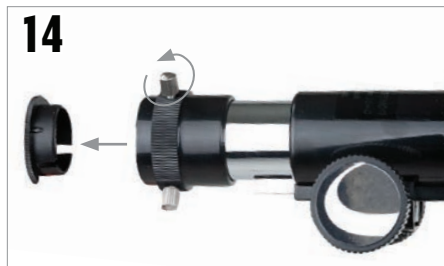
14 Loosen the set screws on the focuser and remove the plastic cap.
