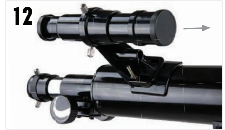
12 Orient the finderscope so that it is facing towards the front of the tube. Place the finderscope over the screws as shown.
