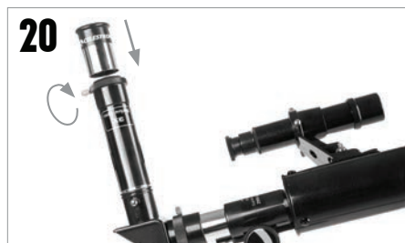
20 Insert the barrel of the 20mm eyepiece into the Barlow lens and tighten the screws to secure it in place.
