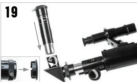
19 For additional magnification, you can use the included 3x Barlow lens. Place the Barlow lens in the focuser in place of the eyepiece. Remove the cap from the Barlow lens.
