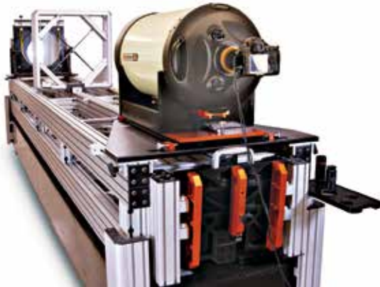
FIGURE 12. In the Final Acceptance Test, the EdgeHD optics must demonstrate the ability to form sharp images at the center and in the corners of a full-frame digital SLR camera, with a sensor that measures 42mm corner-to-corner.
