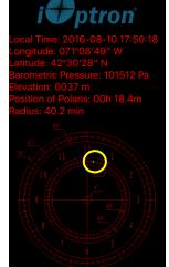
Press the power switch on the mount to turn on the mount. Look through the polar scope eyepiece. If you can not see red polar scope dial or a large tick mark is not on top, release RA Clutch Disk slightly. Rotate the RA axis until you see the red LED illumination and/or adjust one of the large tick makr to the top. Lock the RA axis again. Adjust the eyepiece to bring the reticle dial in focus.
